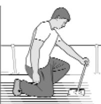
1. Install your pump where you can pump comfortably - particularly important in an emergency when prolonged periods of pumping may be necessary.
