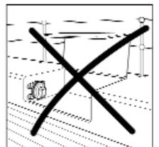
2. Avoid installations which require you to open a cockpit locker to operate the pump
