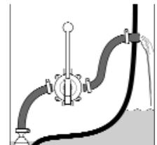
3. Ideally, for minimum pumping effort you should site the pump halfway in height between strainer box and hull outlet
