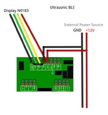
2. Connection from the Calypso Instruments Portable Range. 2.2 How to connect the Calypso Instruments Portable Range via Bluetooth to the NCP High-End via cable to an NMEA 0183 display.
