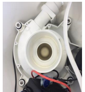
14. Replace waste pump
