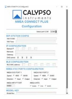
To configure the Portable wind meter to the NCP High-End fill in the following fields:
